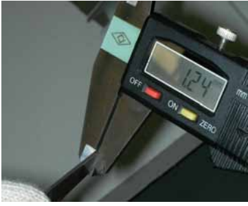
Thickness of the steel
